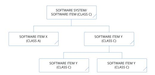
*Figure 1: Example of decomposition of software items according to IEC 62304:2006 +AMD1:2015 Figure B.18*
